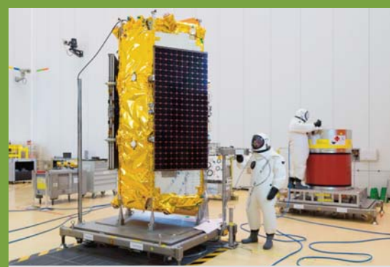
Remplissage d'un des quatre O3b MEO Satellites au CSG One of the four O3b MEO Satellites being filled with propellant at the CSG
